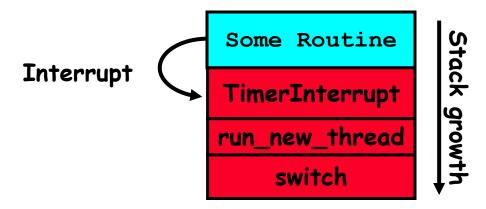
• I/O interrupt: same as timer interrupt except that DoHousekeeping() replaced by ServiceIO().
