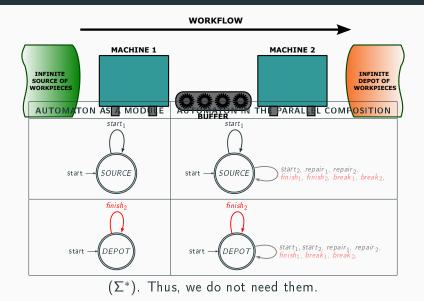
Requirement 1: Machine 1 can start processing a workpiece only if the Buffer is empty
