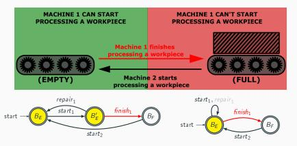
Can Machine 1 be repaired if it didn't even start? (=can we further simplify the requirement?)
