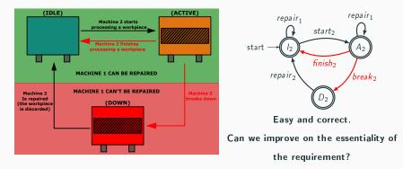
Rationale: When Machine 2 is down if we repair Machine 1 it means that Machine 1 is down as well.
