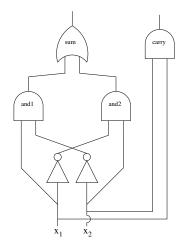
This is the schematic of a **half-adder circuit** that we want to compile into an OBDD. It has the following truth table:
