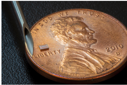
The alcohol monitoring chip alongside a penny and a 16 gauge needle. Photos by David Baillot/ UC San Diego Jacobs School of Engineering.
